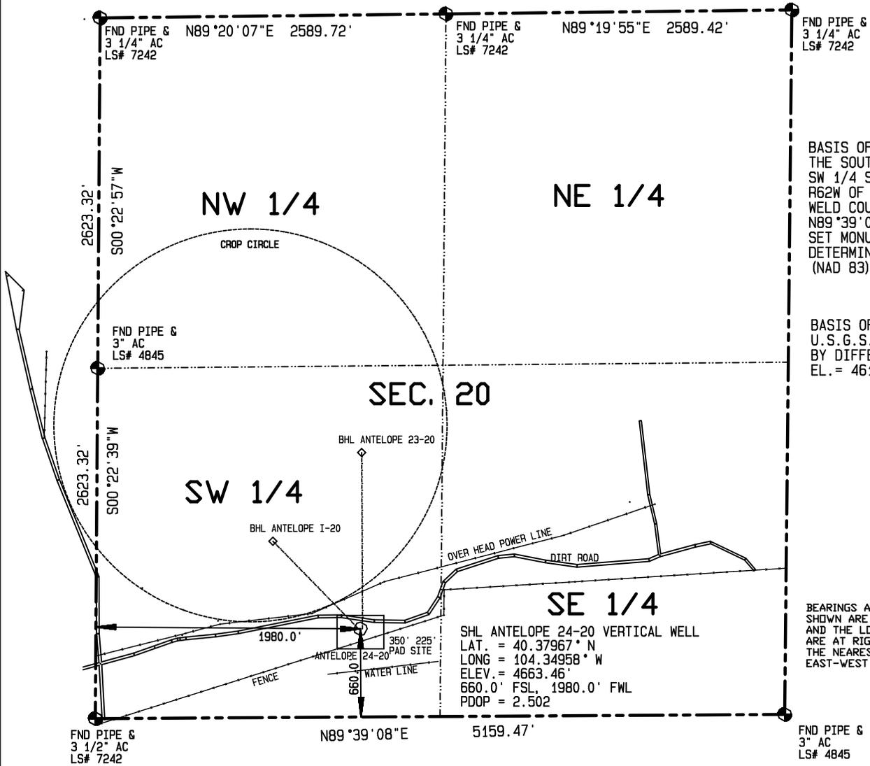
BASIS OF BEARINGS IS THE SOUTH LINE OF THE SW 1/4 SEC. 20, T5N, R62W OF THE 6TH P.M. WELD COUNTY, CO. BEARS N89°39'08"E BETWEEN SET MONUMENTS AS DETERMINED BY GPS (NAD 83)
