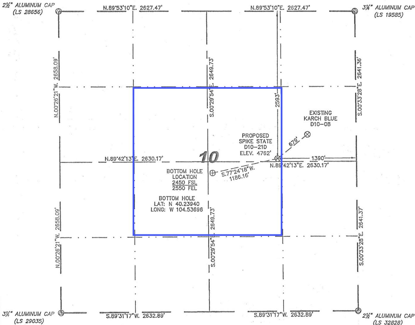
IN ACCORDANCE WITH A REQUEST FROM BRIAN DeROSE - NOBLE ENERGY INC, STELL SURVEYING SERVICES, LLC HAS DETERMINED THE LOCATION OF THE SPIKE STATE D10-21D WELL TO BE 2593' FNL, 1390' FEL, AS MEASURED AT NINETY (90) DEGREES FROM THE SECTION LINES, SECTION 10, TOWNSHIP 3 NORTH, RANGE 64 WEST, 6TH PRINCIPLE MERIDIAN, WELD COUNTY, COLORADO.
