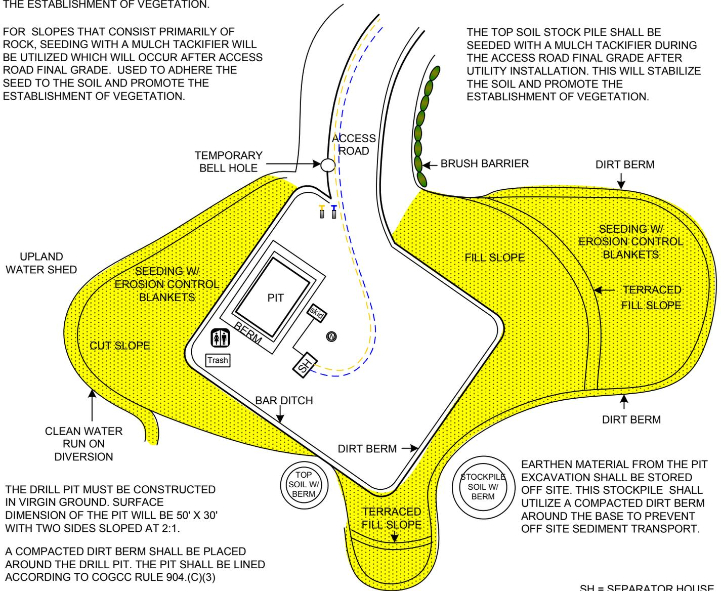
THE DRILL PIT MUST BE CONSTRUCTED IN VIRGIN GROUND. SURFACE DIMENSION OF THE PIT WILL BE 50' X 30' WITH TWO SIDES SLOPED AT 2:1.
