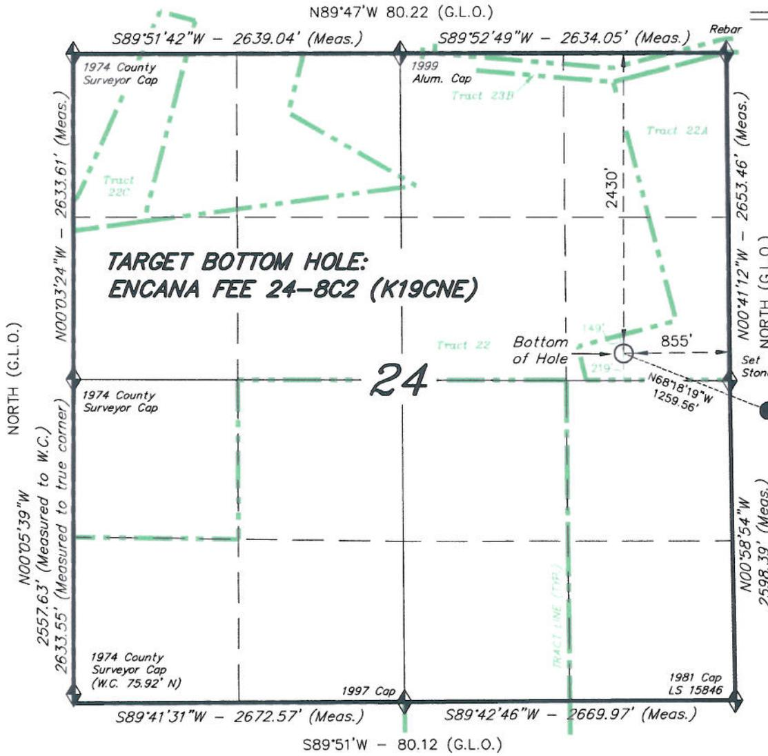
TARGET BOTTOM HOLE, ENCANA FEE 24-8C2 (K19CNE), LOCATED AS SHOWN IN THE SE 1/4 NE 1/4 OF SECTION 24, T6S, R93W, 6th P.M. GARFIELD COUNTY, COLORADO.
