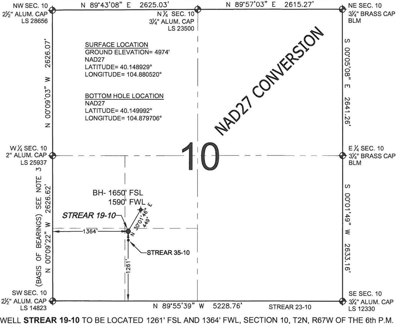
WELL **STREAR 19-10** TO BE LOCATED 1261' FSL AND 1364' FWL, SECTION 10, T2N, R67W OF THE 6th P.M.
