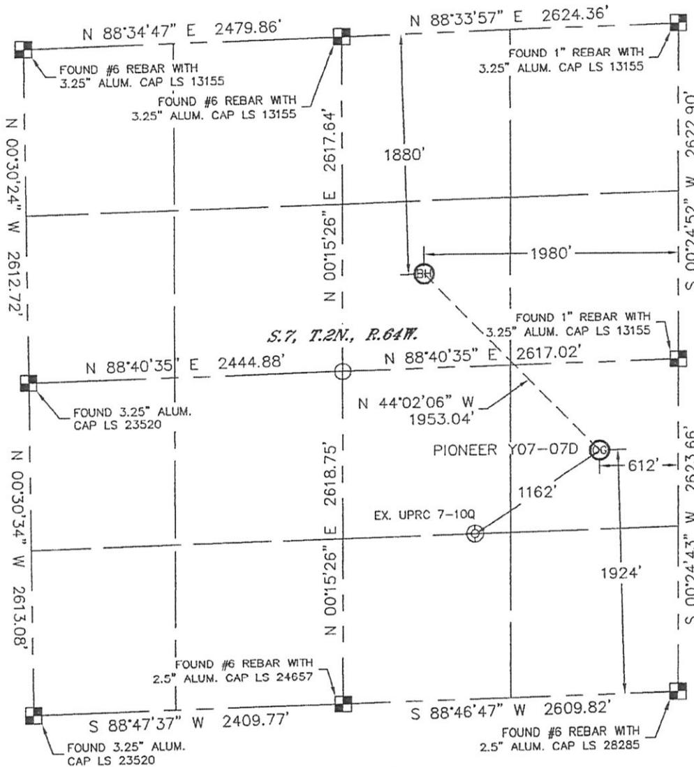
In accordance with a request from CJ Pietri with Noble Energy Inc. Lat40°, Inc. has determined the surface location of the PIONEER Y07-07D to be 1924' from the SOUTH line and 612' from the EAST line and the bottom hole to be 1880' from the NORTH line and 1980' from the EAST line as measured at right angles from the section lines of Section 7, Township 2 North, Range 64 West of the Sixth Principal Meridian, County of Weld, State of Colorado.
