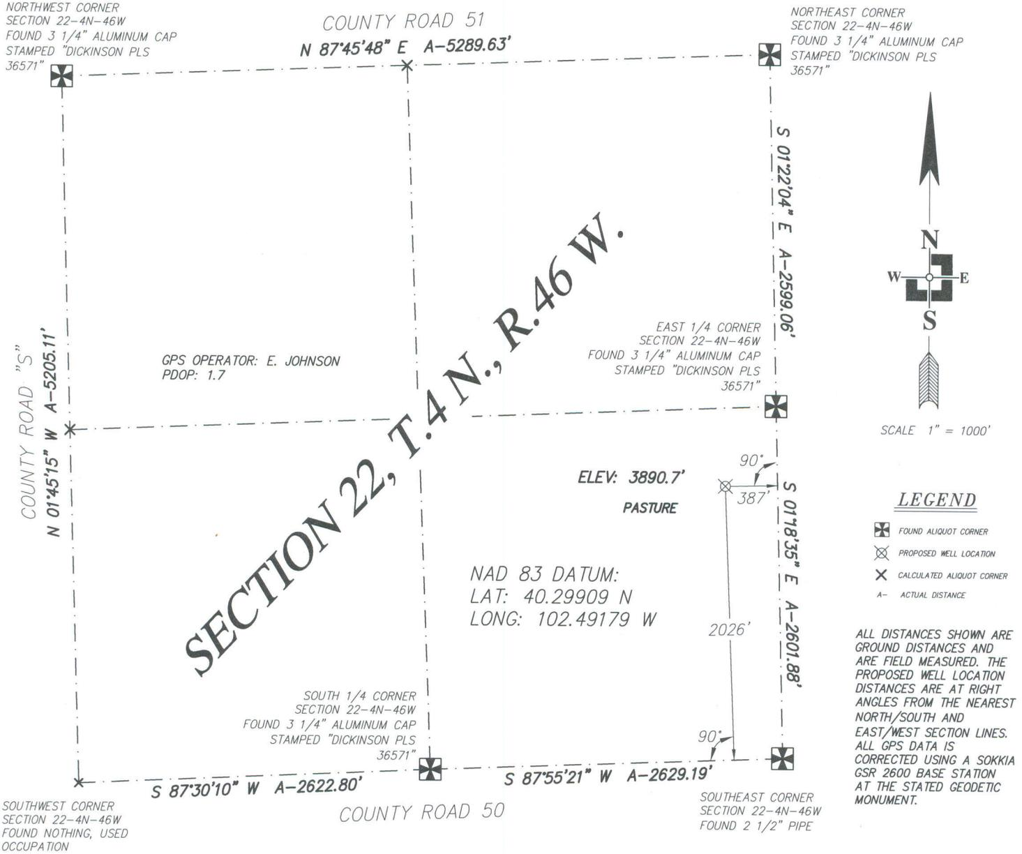
ALL DISTANCES SHOWN ARE GROUND DISTANCES AND ARE FIELD MEASURED. THE PROPOSED WELL LOCATION DISTANCES ARE AT RIGHT ANGLES FROM THE NEAREST NORTH/SOUTH AND EAST/WEST SECTION LINES. ALL GPS DATA IS CORRECTED USING A SOKKIA GSR 2600 BASE STATION AT THE STATED GEODETIC MONUMENT.
