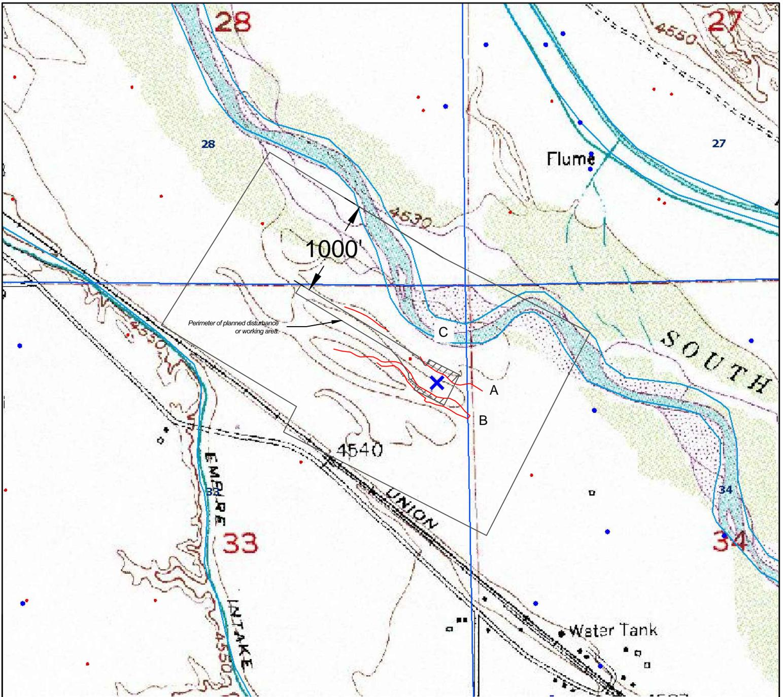
Silt Fencing will be installed to prevent sedimentation of delineated wet areas (hatched area on drawing), prior to construction of drilling pad. Delineated wet areas will not receive any fill during construction or operation of the pad.
