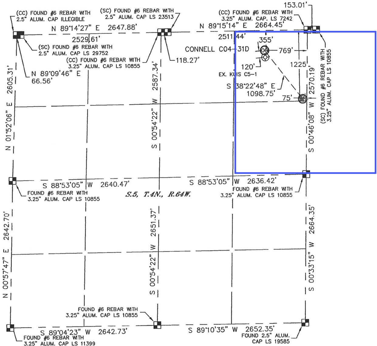
In accordance with a request from CJ Pietri with Noble Energy Inc., Lat40°, Inc. has determined the surface location of the CONNELL C04-31D to be 355' from the NORTH line and 769' from the EAST line and the bottom hole to be 1225' from the NORTH line and 75' from the EAST line as measured at right angles from the section lines of Section 5, Township 4 North, Range 64 West of the Sixth Principal Meridian, County of Weld, State of Colorado.
