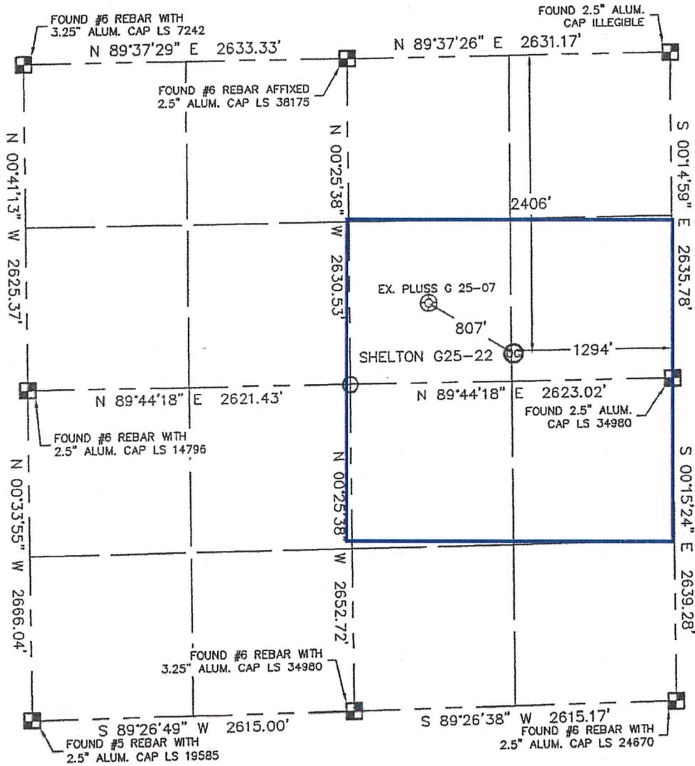
In accordance with a request from Beau Fritz with Noble Energy Inc. Lat40°, LLC has determined the surface location of the SHELTON G25-22 to be 2406' from the NORTH line and 1294' from the EAST line as measured at right angles from the section lines of Section 25, Township 4 North, Range 65 West of the Sixth Principal Meridian, County of Weld, State of Colorado.
