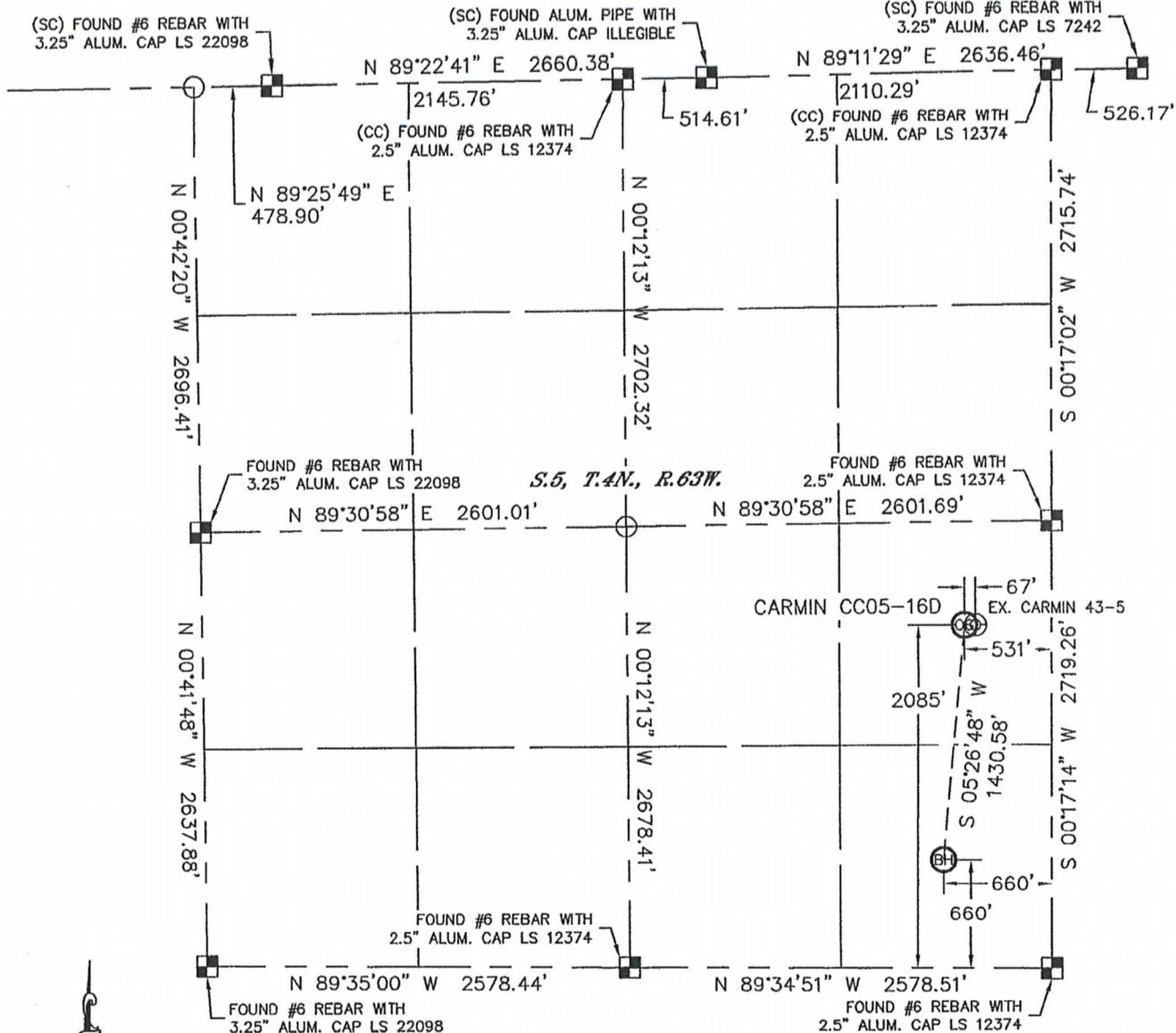
In accordance with a request from Nate McCorkell with Noble Energy Inc. Lat40°, Inc. has determined the surface location of the CARMIN CC05-16D to be 2085' from the SOUTH line and 531' from the EAST line and the bottom hole to be 660' from the SOUTH line and 660' from the EAST line as measured at right angles from the section lines of Section 5, Township 4 North, Range 63 West of the Sixth Principal Meridian, County of Weld, State of Colorado.
