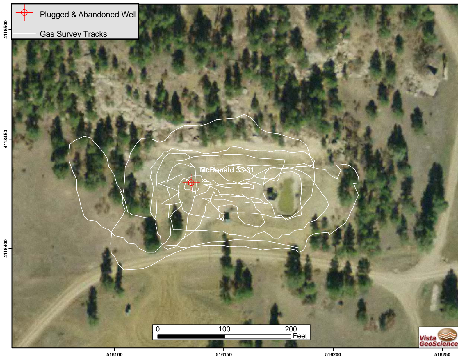
Figure 18. Distribution of gas survey tracks over and around the McDonald plugged & abandoned well. Ground surface methane seeps were not detected over the 1 mile-long track.
