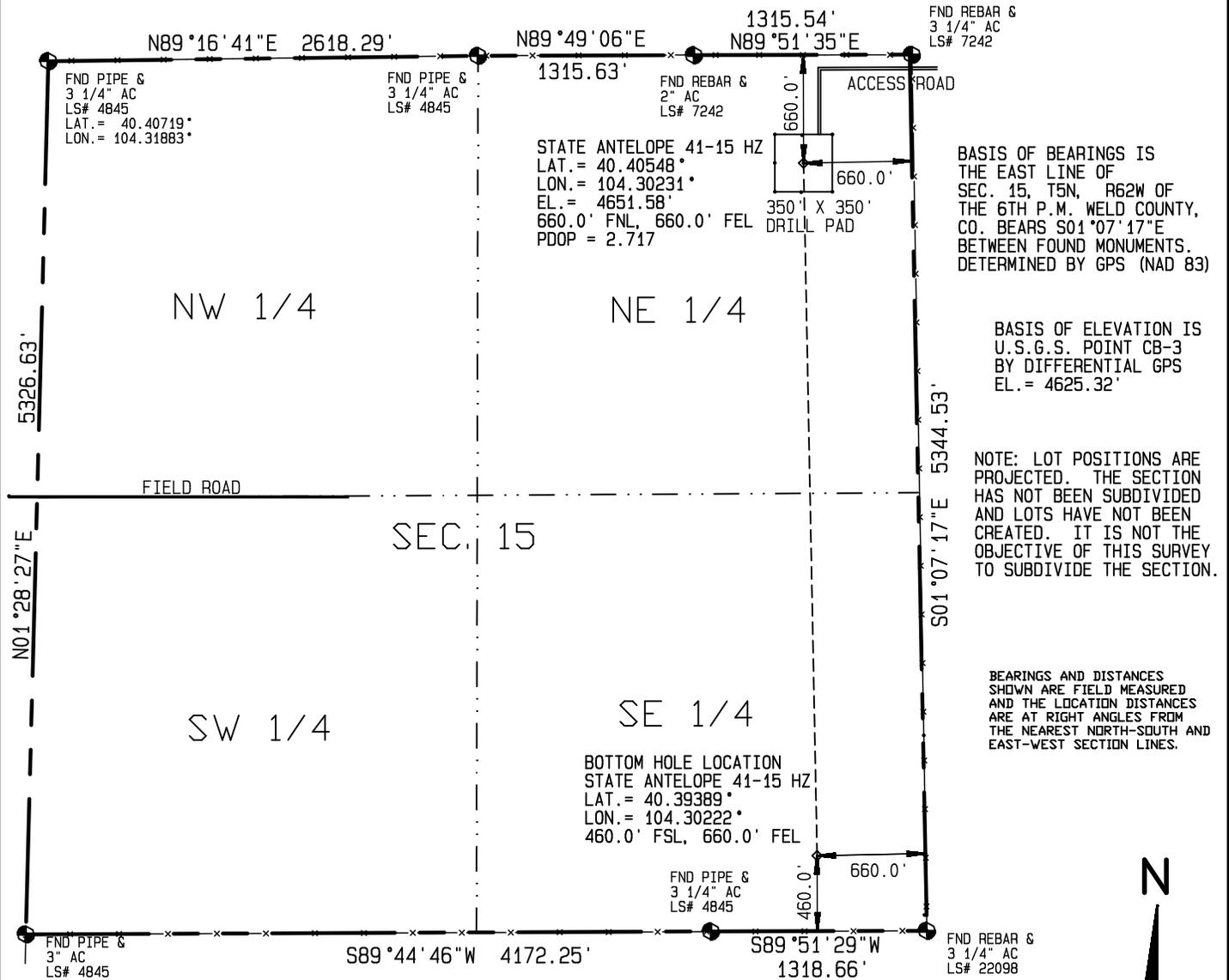
BASIS OF BEARINGS IS THE EAST LINE OF SEC. 15, T5N, R62W OF THE 6TH P.M. WELD COUNTY, CO. BEARS S01°07'17"E BETWEEN FOUND MONUMENTS. DETERMINED BY GPS (NAD 83)
