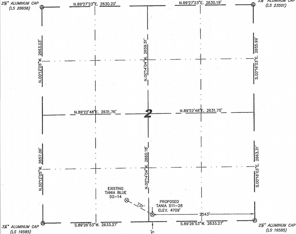
IN ACCORDANCE WITH A REQUEST FROM BRIAN DORSE - NOBLE ENERGY INC, STEIL SURVEYING SERVICES, LLC HAS DETERMINED THE LOCATION OF THE TANIA D11-28 WELL TO BE 175' FSL, 2543' FEL, AS MEASURED AT NINETY (90) DEGREES FROM THE SECTION LINES, SECTION 2, TOWNSHIP 3 NORTH, RANGE 64 WEST, 6TH PRINCIPLE MERIDIAN, WELD COUNTY, COLORADO.
