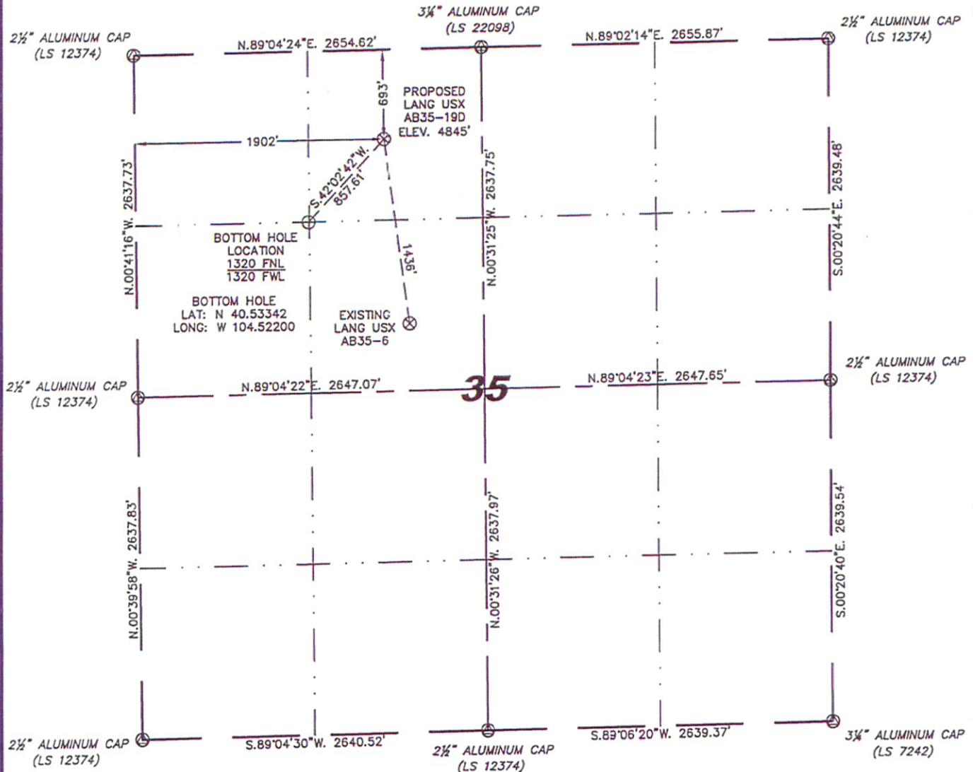
IN ACCORDANCE WITH A REQUEST FROM RYAN ANTONIO - NOBLE ENERGY INC, STEIL SURVEYING SERVICES, LLC HAS DETERMINED THE LOCATION OF THE LANG USX AB35-19D WELL TO BE 693' FNL, 1902' FWL, AS MEASURED AT NINETY (90) DEGREES FROM THE SECTION LINES, SECTION 35, TOWNSHIP 7 NORTH, RANGE 64 WEST, 6TH PRINCIPLE MERIDIAN, WELD COUNTY, COLORADO.
