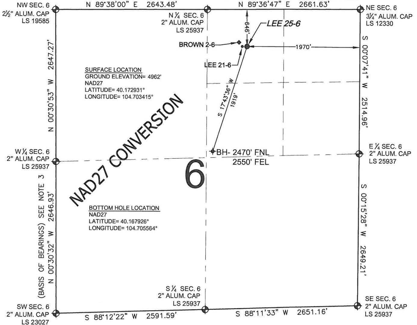
WELL LEE 25-6 TO BE LOCATED 646' FNL AND 1970' FEL, SECTION 6, T2N, R65W OF THE 6th P.M.
