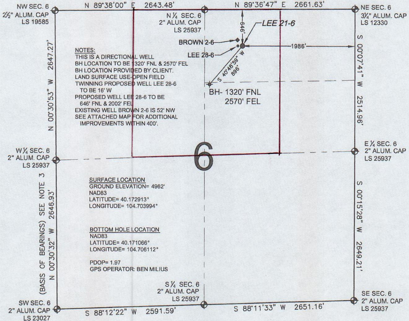
WELL LEE 21-6 TO BE LOCATED 646' FNL AND 1986' FEL, SECTION 6, T2N, R65W OF THE 6th P.M.
