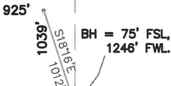
I HEREBY STATE TO UNIOIL THAT THIS WELL LOCATION CERTIFICATE FOR THE WELL ZEILER 7LDU IS LOCATED 1039' FSL & 925' FWL, SEC. 7, T5N, R67W, 6PM.
