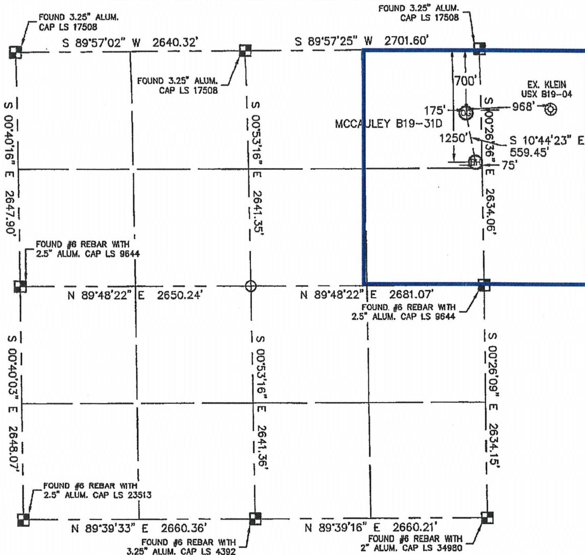
In accordance with a request from Matt Campbell with Noble Energy Inc., Lat40°, LLC has determined the surface location of the MCCAULEY B19-31D to be 700' from the NORTH line and 175' from the EAST line and the bottom hole to be 1250' from the NORTH line and 75' from the EAST line as measured at right angles from the section line of Section 24, Township 5 North, Range 65 West of the Sixth Principal Meridian, County of Weld, State of Colorado.
