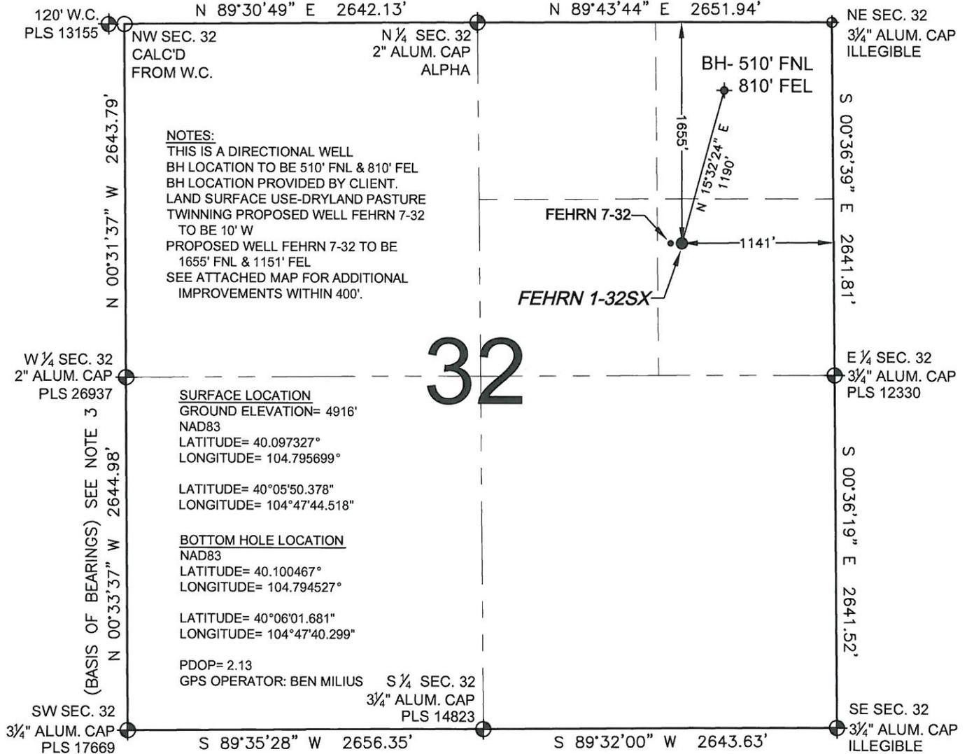
WELL **FEHRN 1-32SX** TO BE LOCATED 1655' FNL AND 1141' FEL, SECTION 32, T2N, R66W OF THE 6th P.M.
