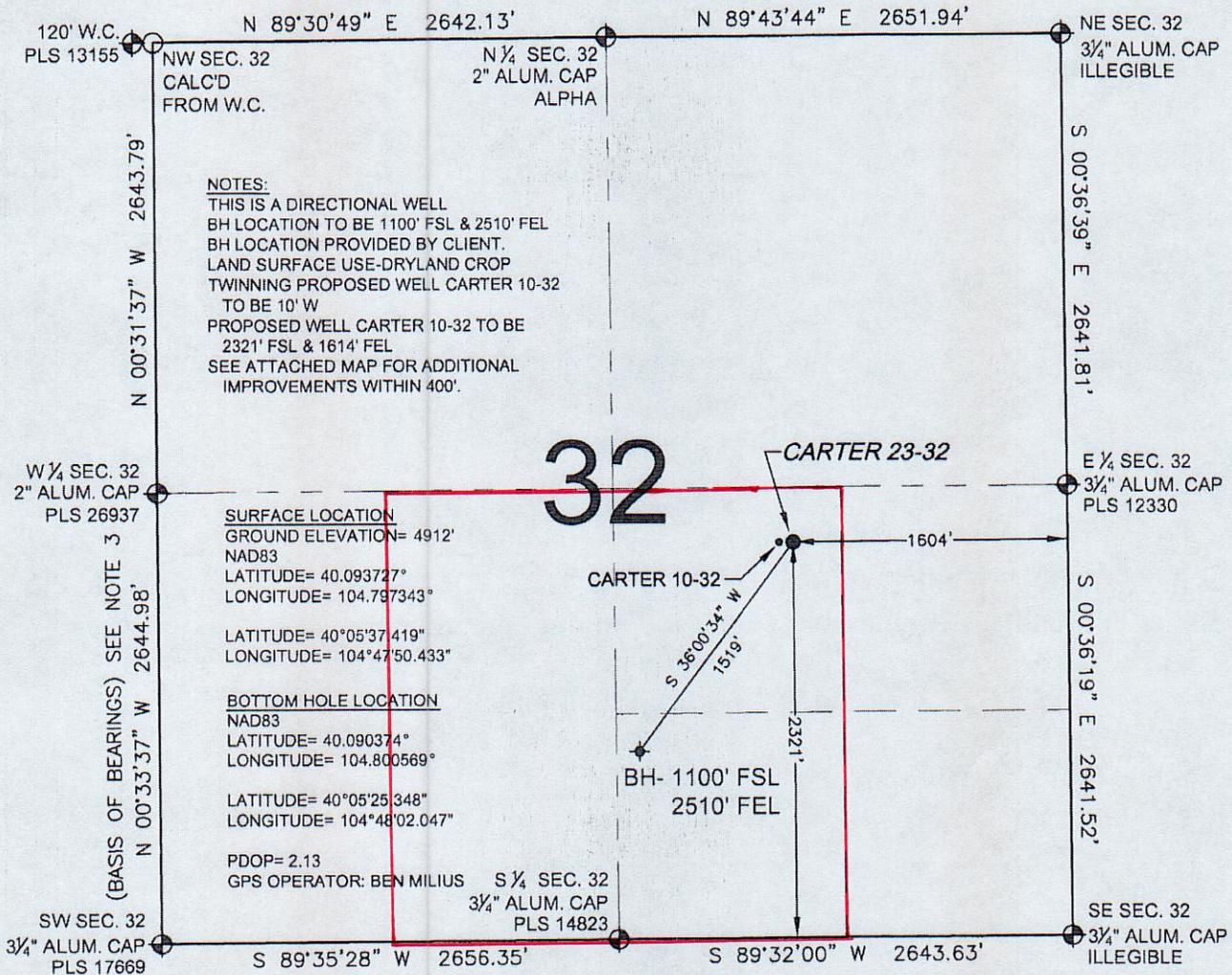
WELL **CARTER 23-32** TO BE LOCATED 2321' FSL AND 1604' FEL, SECTION 32, T2N, R66W OF THE 6th P.M.
