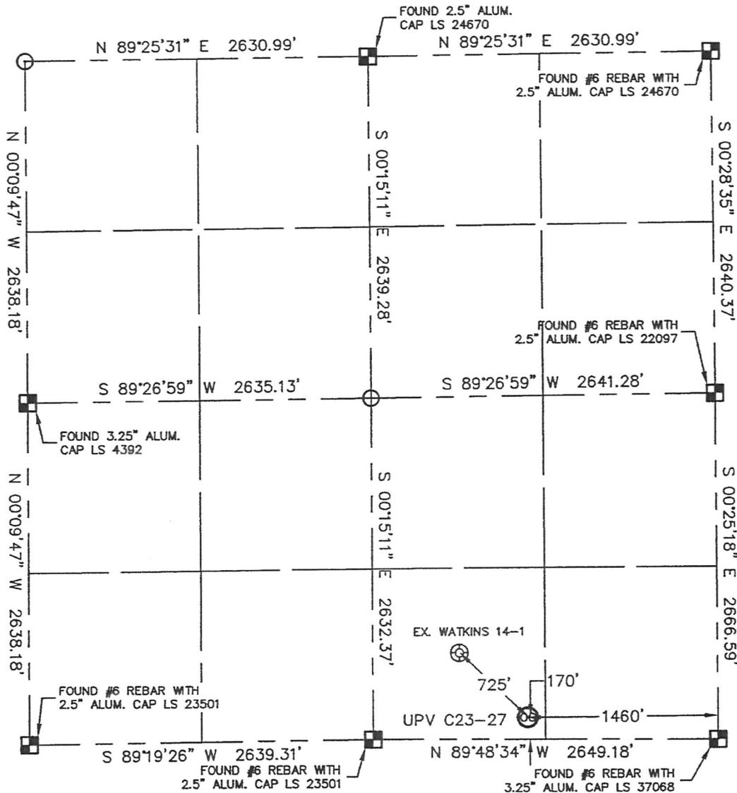
In accordance with a request from MATT CAMPBELL with Noble Energy Inc. Lat40°, LLC has determined the surface location of the UPV C23-27 to be 170' from the SOUTH line and 1460' from the EAST line as measured at right angles from the section line of Section 14, Township 4 North, Range 64 West of the Sixth Principal Meridian, County of Weld, State of Colorado.
