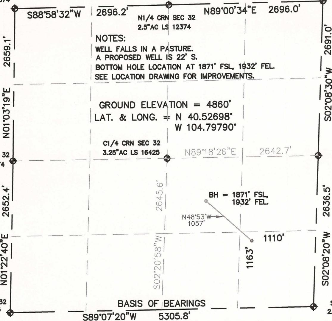
I HEREBY STATE TO PETROLEUM DEVELOPMENT CORP. THAT THIS WELL LOCATION CERTIFICATE FOR THE WELL NELSON 33-32D IS LOCATED 1163' FSL & 1110' FEL, SEC. 32, T7N, R66W, 6PM.
