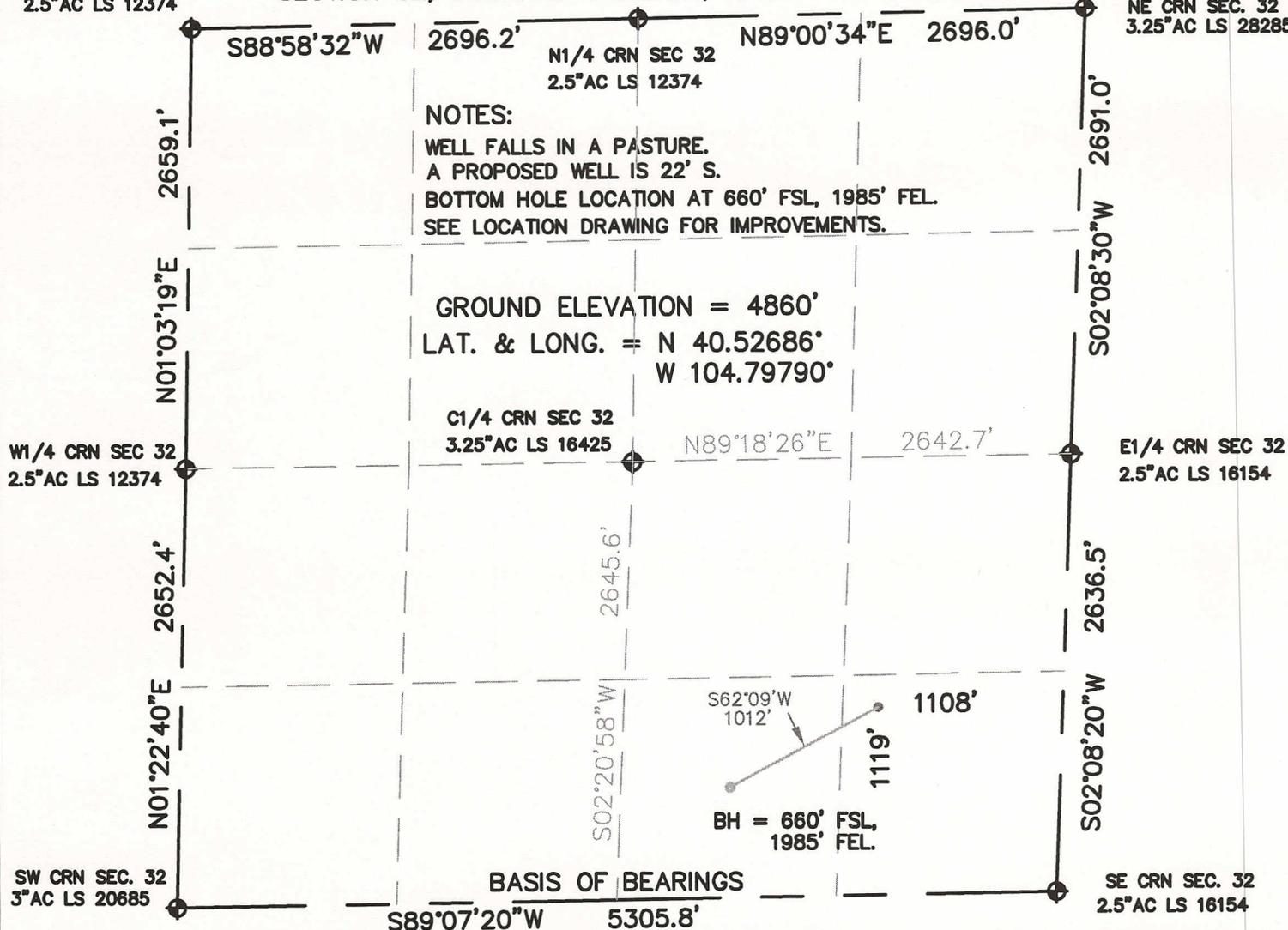
I HEREBY STATE TO PETROLEUM DEVELOPMENT CORP. THAT THIS WELL LOCATION CERTIFICATE FOR THE WELL NELSON 34-32D IS LOCATED 1119' FSL & 1108' FEL, SEC. 32, T7N, R66W, 6PM.
