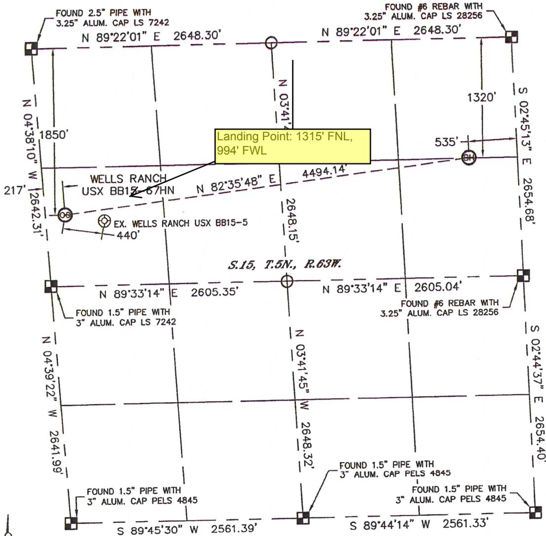
In accordance with a request from Sean Casper with Noble Energy Inc. Lat40°, LLC has determined the surface location of the WELLS RANCH USX BB15-67HN to be 1850' from the NORTH line and 217' from the WEST line and the bottom hole to be 1320' from the NORTH line and 535' from the EAST line as measured at right angles from the section lines of Section 15, Township 5 North, Range 63 West of the Sixth Principal Meridian, County of Weld, State of Colorado.
