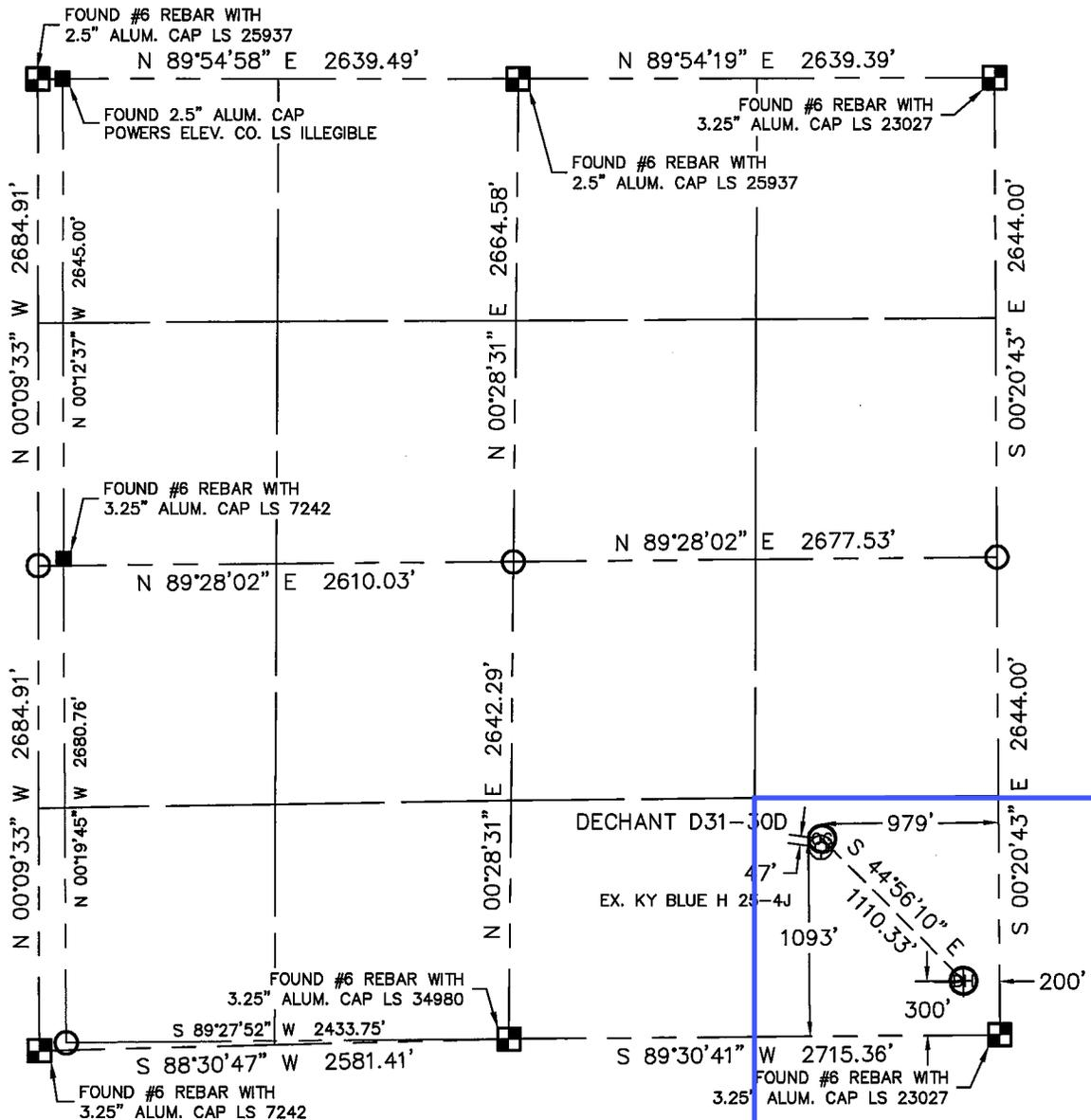
In accordance with a request from CJ PIETRI with Noble Energy Inc. Lat40°, LLC has determined the surface location of the DECHANT D31-300 to be 1093' from the SOUTH line and 979' from the EAST line and the bottom hole to be 300' from the SOUTH line and 200' from the EAST line as measured at right angles from the section lines of Section 25, Township 3 North, Range 65 West of the Sixth Principal Meridian, County of Weld, State of Colorado.
