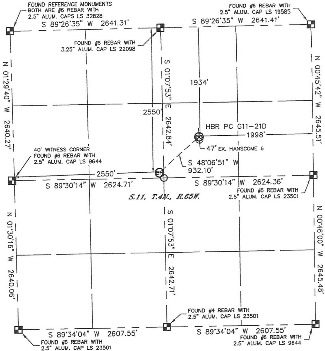
In accordance with a request from Beau Fritz with Noble Energy Inc. Lat40°, LLC has determined the surface location of the HBR PC G11-21D to be 1934' from the NORTH line and 1998' from the EAST line and the bottom hole to be 2550' from the NORTH line and 2550' from the WEST line as measured at right angles from the section lines of Section 11, Township 4 North, Range 65 West of the Sixth Principal Meridian, County of Weld, State of Colorado.
