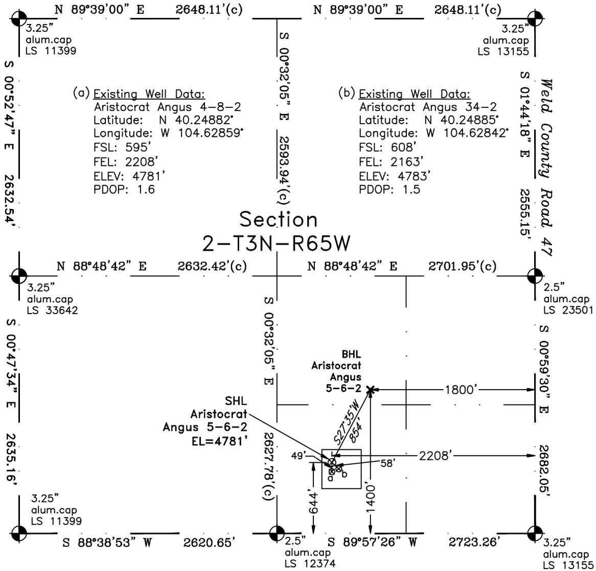
In accordance with a request from Dave Bale of EnCana Oil & Gas (USA) Inc., PLS Group, LLC has determined the location of the Aristocrat Angus 5-6-2 well site to be SHL: 644' FSL and 2208' FEL, (BHL 1400' FSL and 1800' FEL) as measured at ninety (90) degrees from the section lines of Section 2, Township 3 North, Range 65 West, 6th Principal Meridian, County of Weld, CO.
