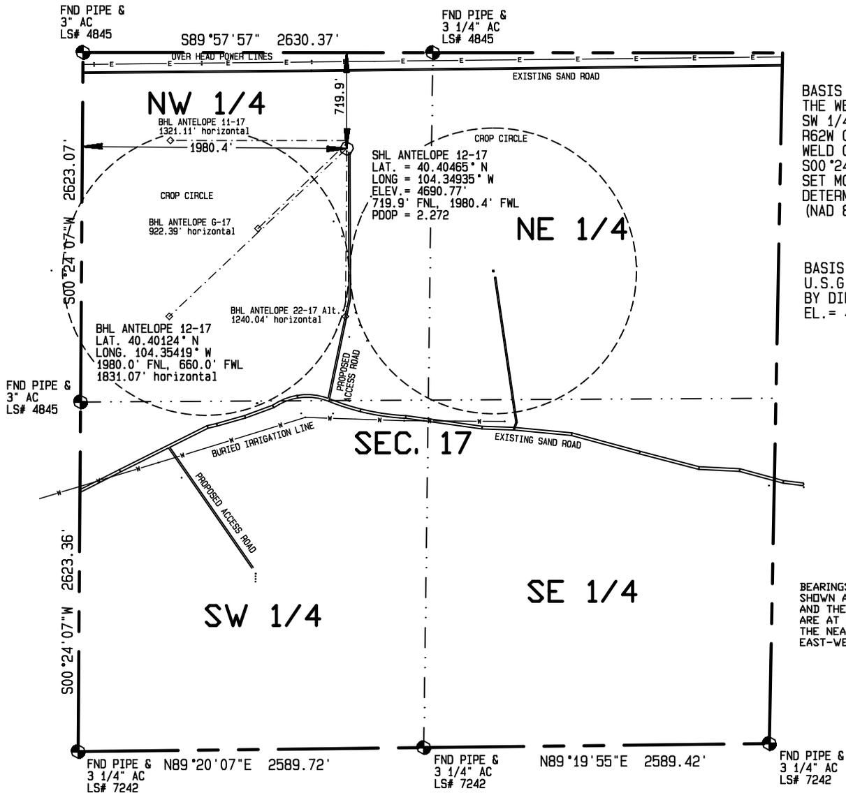
BASIS OF BEARINGS IS THE WEST LINE OF THE SW 1/4 OF SEC. 17, T5N, R62W OF THE 6TH P.M. WELD COUNTY, CO. BEARS S00°24'07\"W BETWEEN SET MONUMENTS AS DETERMINED BY GPS (NAD 83)
