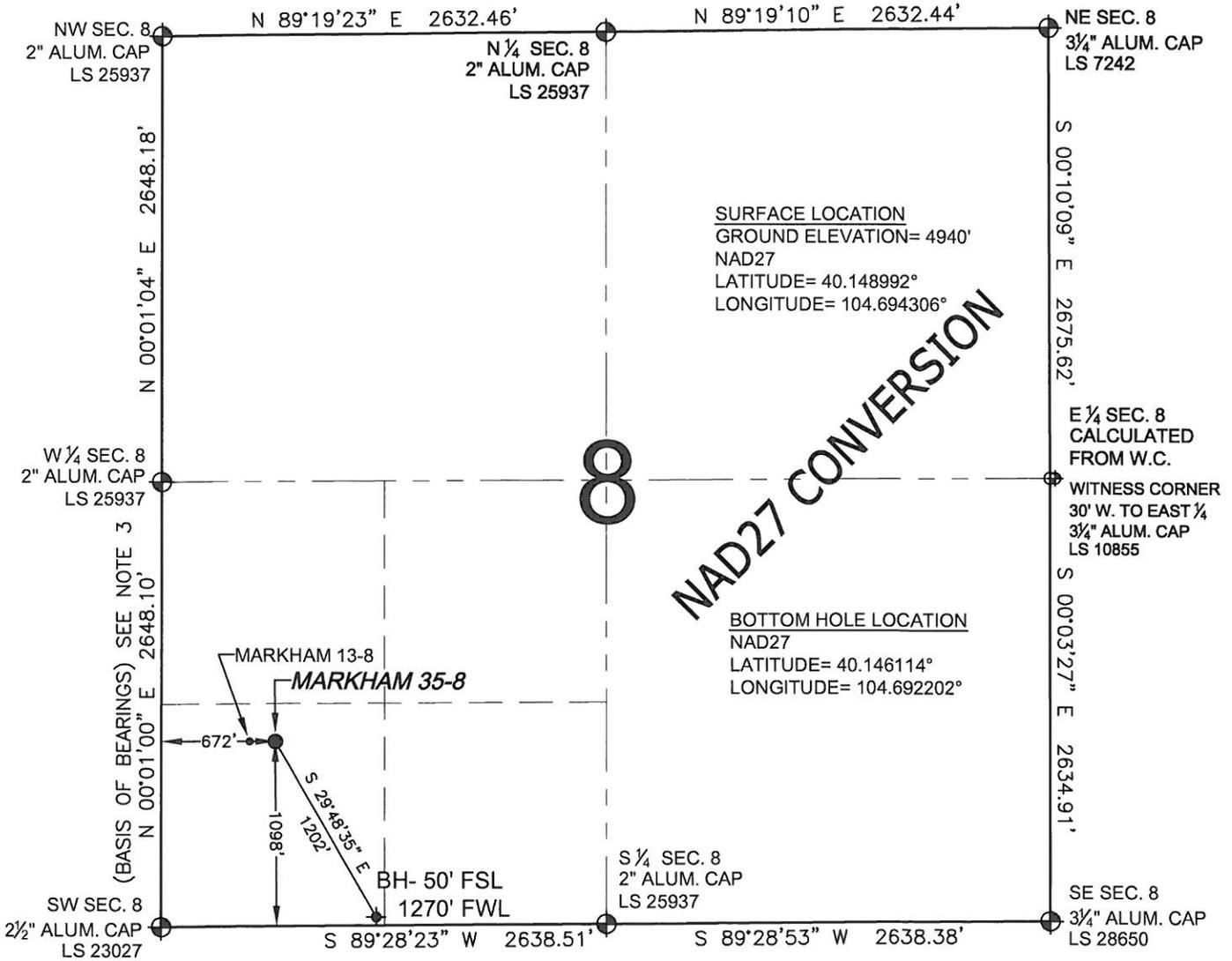
WELL **MARKHAM 35-8** TO BE LOCATED 1098' FSL AND 672' FWL, SECTION 8, T2N, R65W OF THE 6th P.M.
