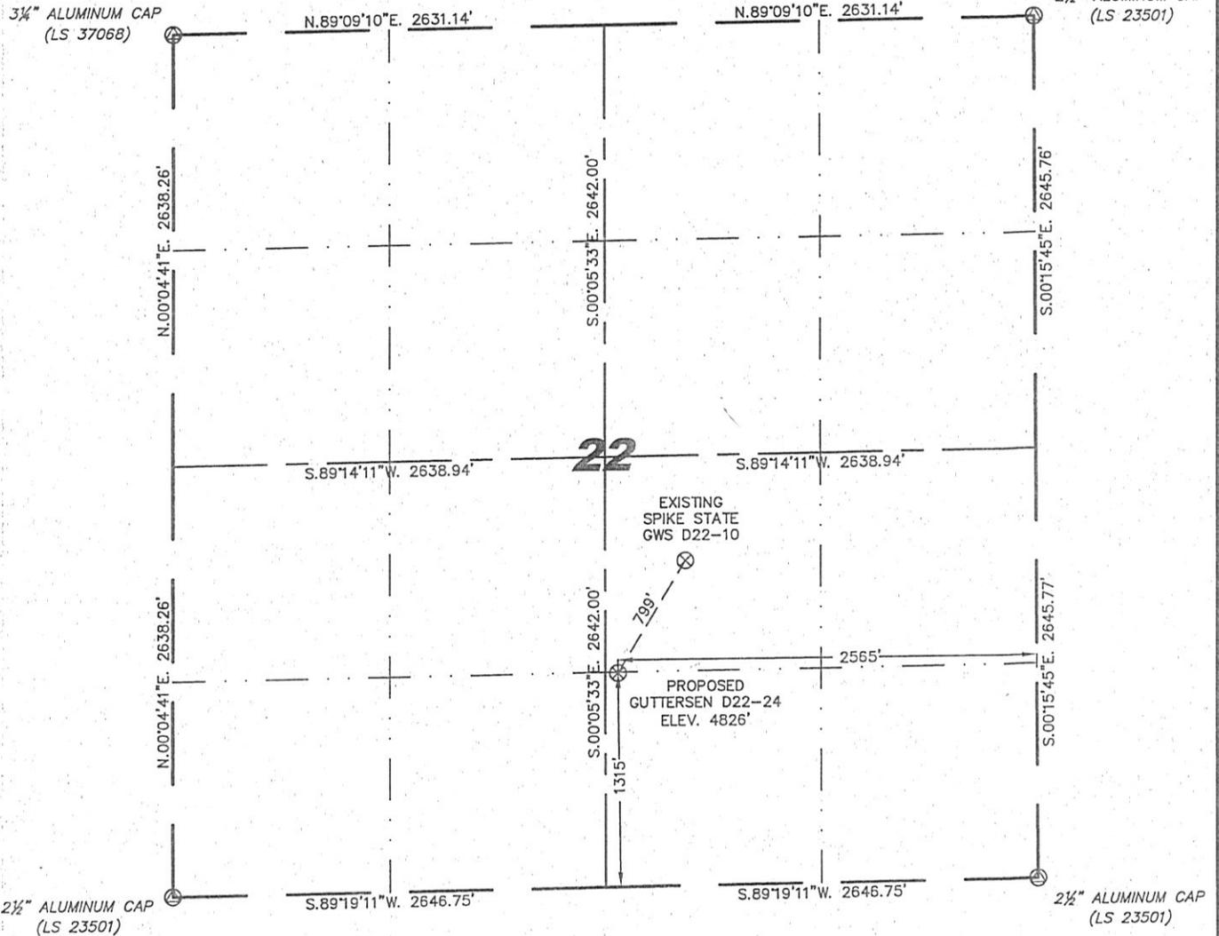
IN ACCORDANCE WITH A REQUEST FROM JOE JOHNSON - NOBLE ENERGY INC, STEIL SURVEYING SERVICES, LLC HAS DETERMINED THE LOCATION OF THE GUTTERSEN D22-24 WELL TO BE 1315' FSL, 2565' FEL, AS MEASURED AT NINETY (90) DEGREES FROM THE SECTION LINES, SECTION 22, TOWNSHIP 3 NORTH, RANGE 64 WEST, 6TH PRINCIPLE MERIDIAN, WELD COUNTY, COLORADO.
