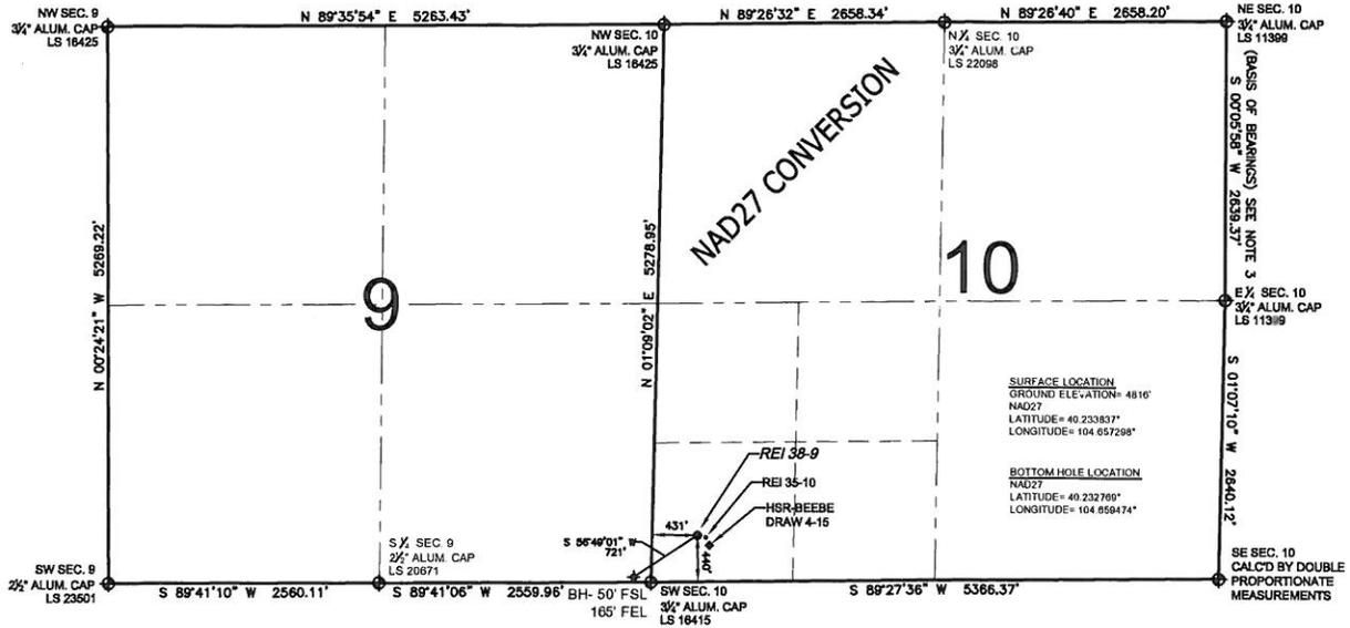
WELL REI 38-9 TO BE LOCATED 440' FSL AND 431' FWL, SECTION 10, T3N, R65W OF THE 6th P.M.
