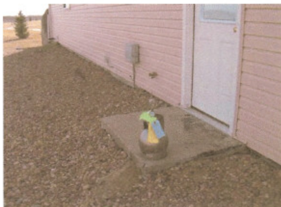
Summa Canister in exterior location on east side of duplex unit
