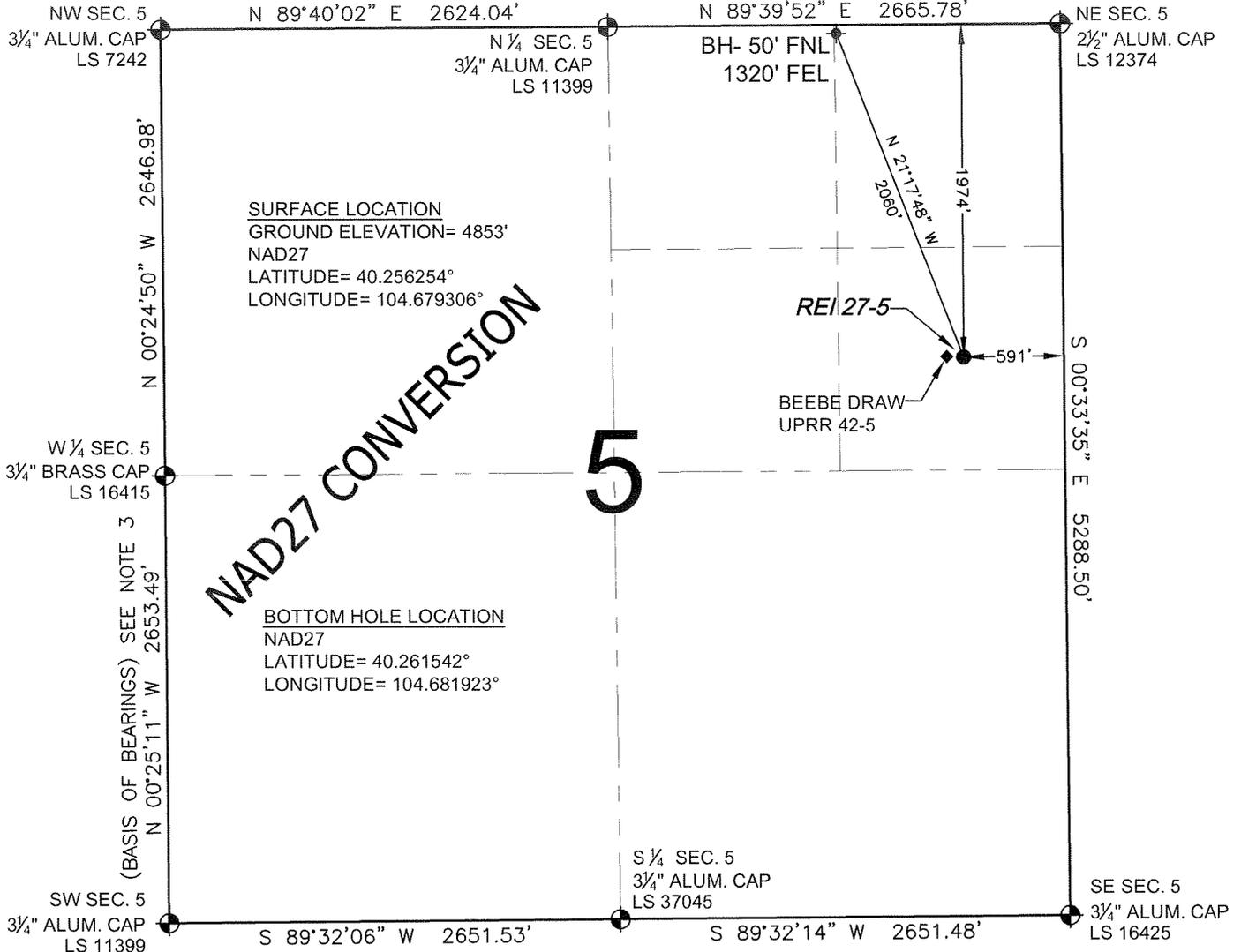
WELL REI 27-5 TO BE LOCATED 1974' FNL AND 591' FEL, SECTION 5, T3N, R65W OF THE 6th P.M.
