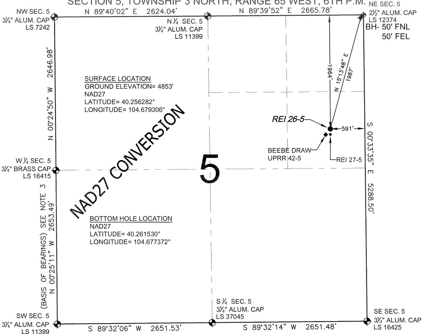
WELL REI 26-5 TO BE LOCATED 1964' FNL AND 591' FEL, SECTION 5, T3N, R65W OF THE 6TH P.M.
