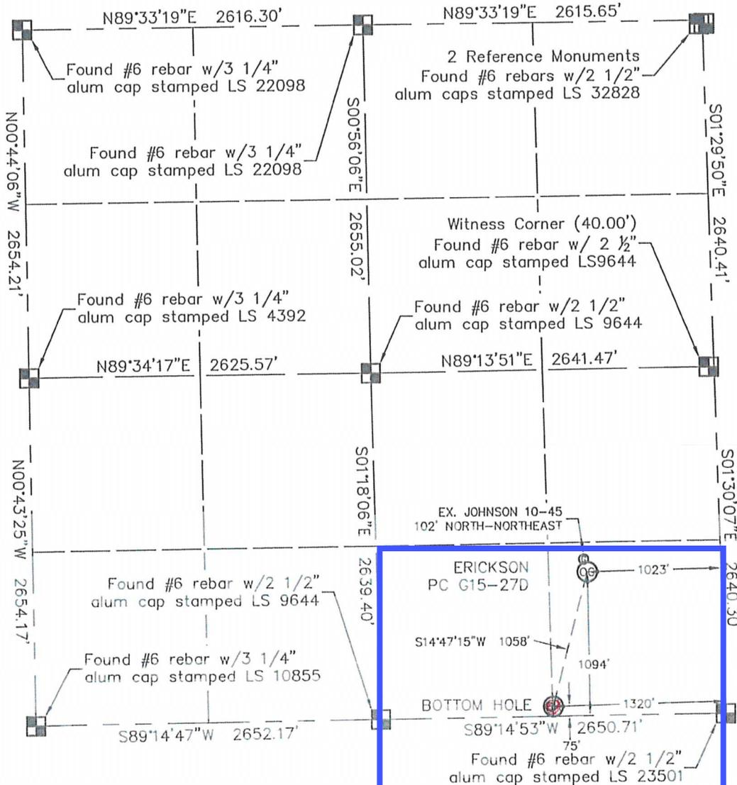
In accordance with a request from BEAU FRITZ with NOBLE ENERGY INC. King Surveyors Inc. has determined the surface location of the ERICKSON PC G15-27D to be 1094' from the South line and 1023' from the East line and the bottom hole to be 75' from the South line and 1320' from the East line, as measured at right angles, from the section lines of Section 10, Township 4 North, Range 65 West of the Sixth Principal Meridian, County of Weld, State of Colorado.
