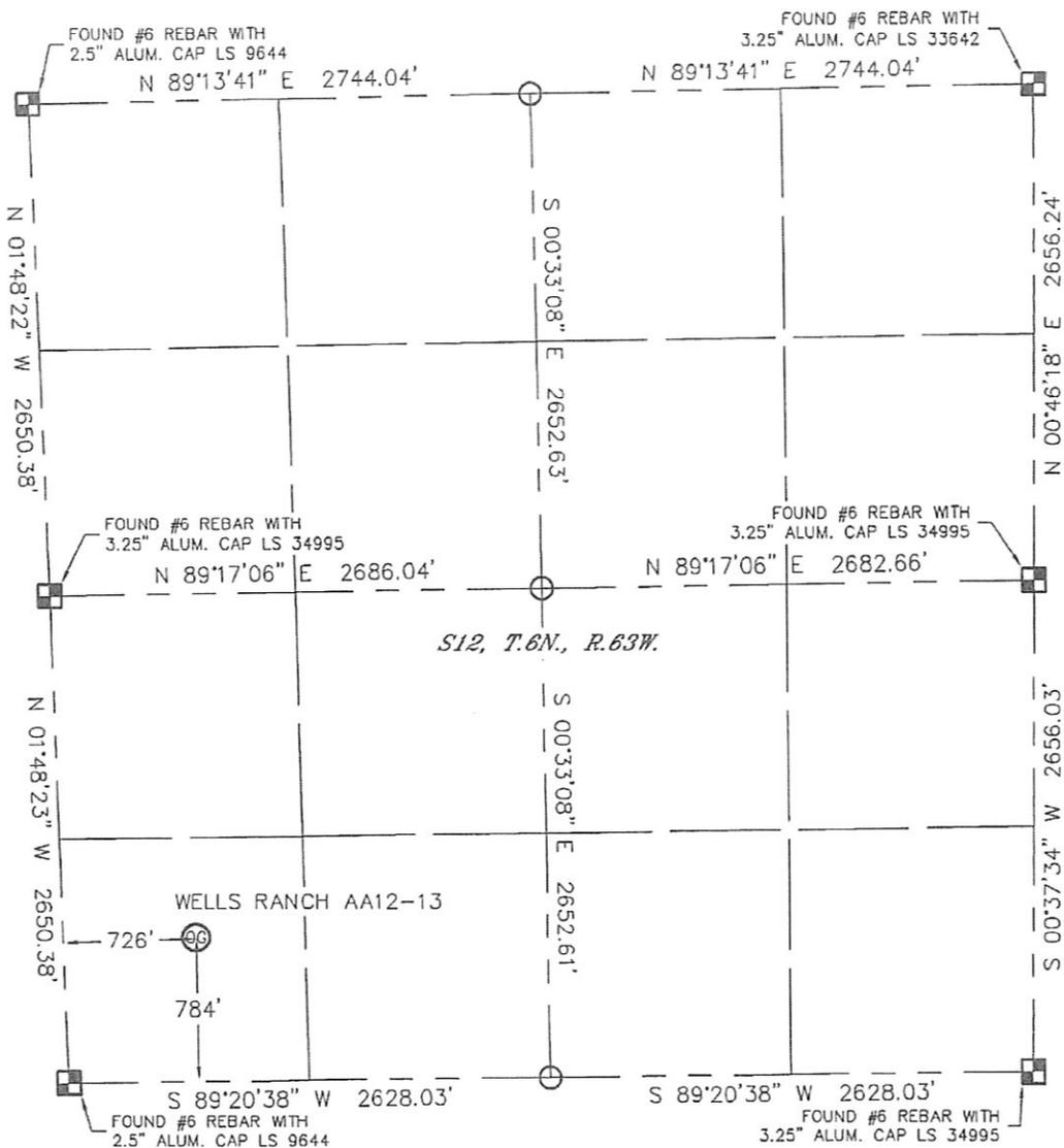
In accordance with a request from Sean Casper with Noble Energy Inc. Lat40°, LLC has determined the surface location of the WELLS RANCH AA12-13 to be 784' from the SOUTH line and 726' from the WEST line as measured at right angles from the section lines of Section 12, Township 6 North, Range 63 West of the Sixth Principal Meridian, County of Weld, State of Colorado.
