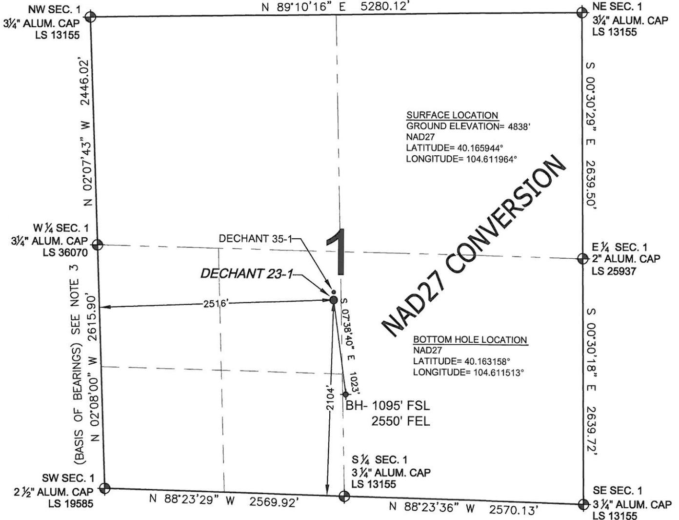
WELL DECHANT 23-1 TO BE LOCATED 2104' FSL AND 2516' FWL, SECTION 1, T2N, R65W OF THE 6TH P.M.
