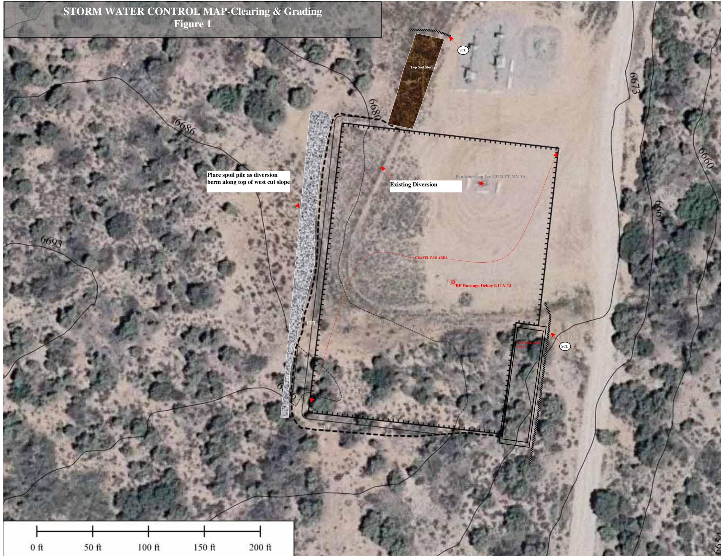
Place spoil pile as diversion berm along top of west cut slope
