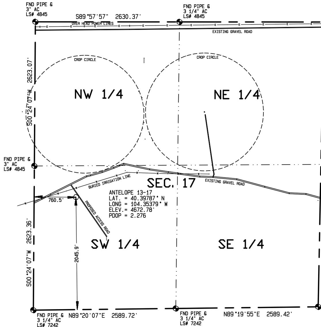
BASIS OF BEARINGS IS THE WEST LINE OF THE SW 1/4 OF SEC. 17, T5N, R62W OF THE 6TH P.M. WELD COUNTY, CO. BEARS S00°24'07\"W BETWEEN SET MONUMENTS AS DETERMINED BY GPS (NAD 83)
