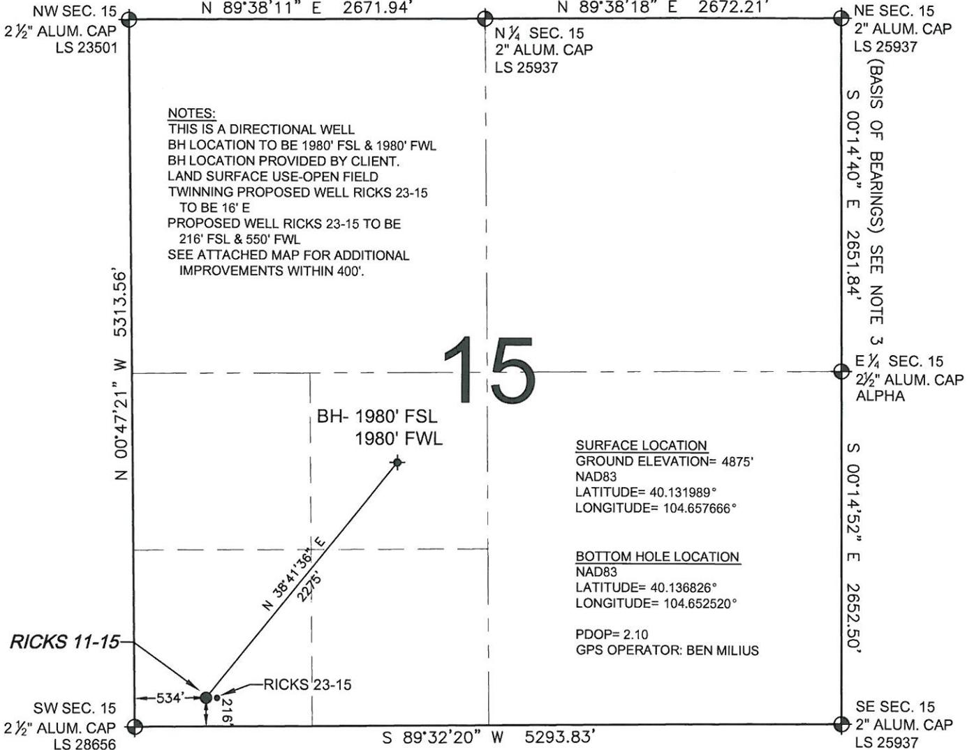
WELL RICKS 11-15 TO BE LOCATED 216' FSL AND 534' FWL, SECTION 15, T2N, R65W OF THE 6th P.M.
