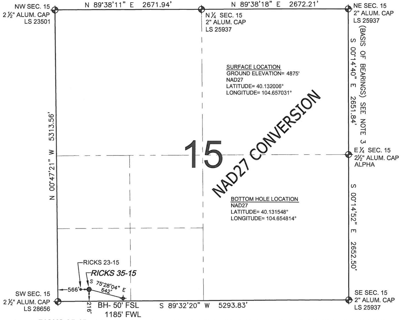
**WELL RICKS 35-15 TO BE LOCATED 216' FSL AND 566' FWL, SECTION 15, T2N, R65W OF THE 6th P.M.**
