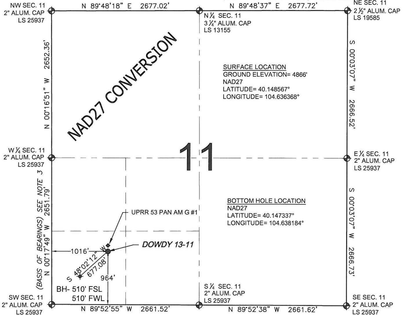
WELL **DOWDY 13-11** TO BE LOCATED 964' FSL AND 1016' FWL, SECTION 11, T2N, R65W OF THE 6th P.M.
