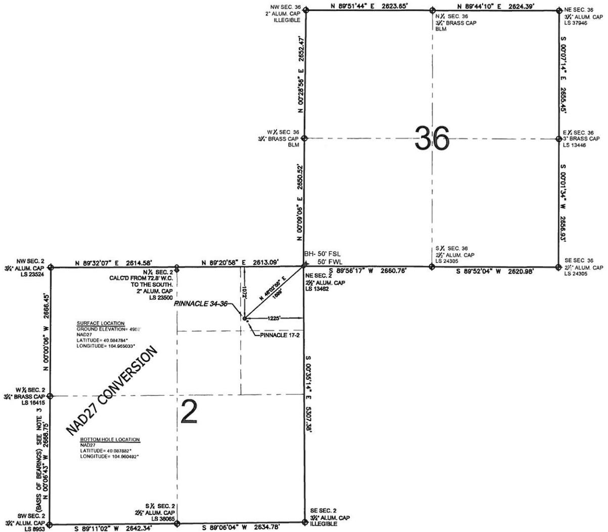
WELL **PINNACLE 34-36** TO BE LOCATED 1072' FNL AND 1225' FEL, SECTION 2, T1N, R68W OF THE 6th P.M.
