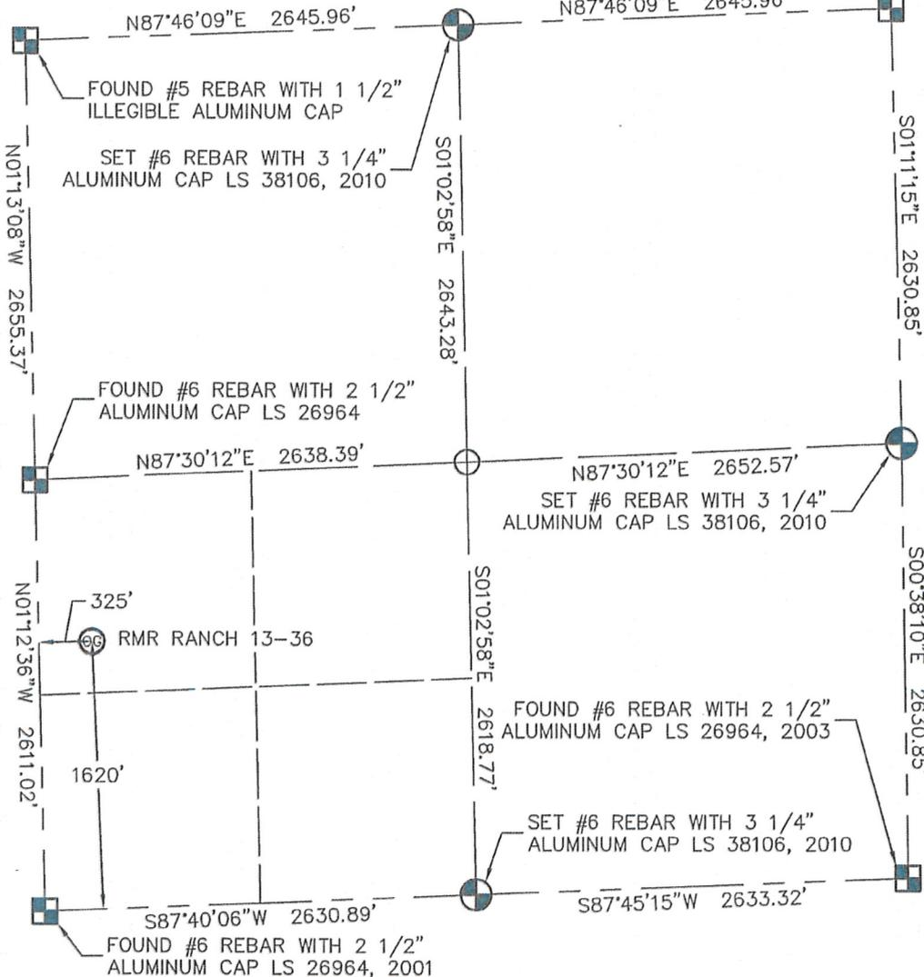
In accordance with a request from DAVID LEDET with NOBLE ENERGY INC. King Surveyors Inc. has determined the surface location of RMR RANCH 13-36 to be 1620' from the SOUTH line and 325' from the WEST line, as measured at right angle, from the section lines of Section 36, Township 2 North, Range 47 West of the Sixth Principal Meridian, County of Yuma, State of Colorado.
