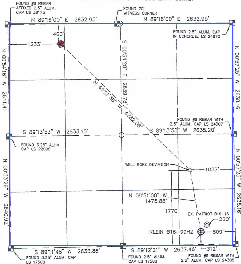
In accordance with a request from Roger Lowe with Noble Energy Inc. Lat40°, LLC has determined the surface location of the KLEIN B16-99HZ to be 312' from the SOUTH line and 809' from the EAST line and the bottom hole to be 460' from the NORTH line and 1233' from the WEST line as measured at right angles from the section line of Section 16, Township 5 North, Range 64 West of the Sixth Principal Meridian, County of Weld, State of Colorado.
