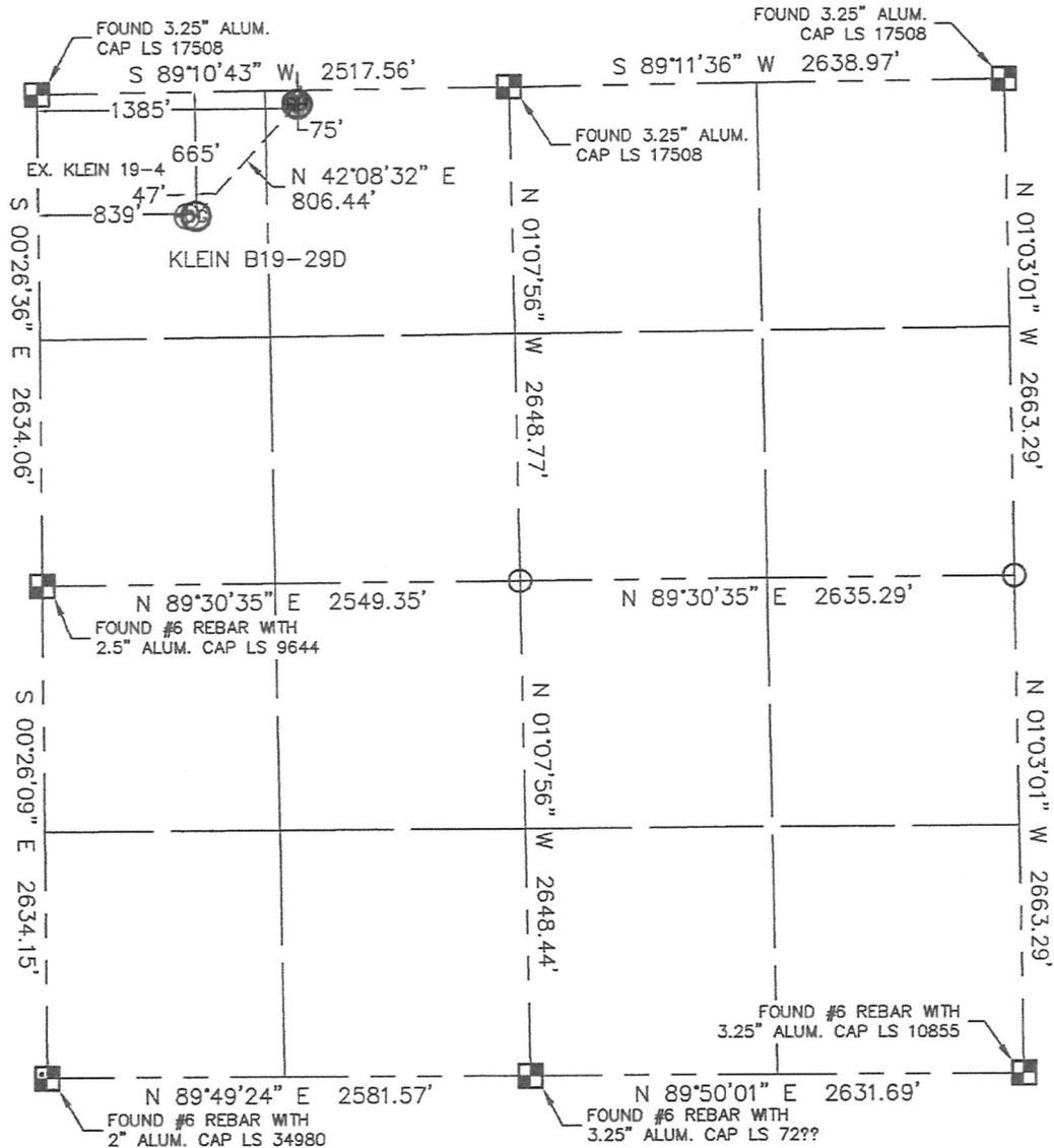
In accordance with a request from Matt Campbell with Noble Energy Inc. Lat40°, LLC has determined the surface location of the KLEIN B19-29D to be 665' from the NORTH line and 839' from the WEST line and the bottom hole to be 75' from the NORTH line and 1385' from the WEST line as measured at right angles from the section line of Section 19, Township 5 North, Range 64 West of the Sixth Principal Meridian, County of Weld, State of Colorado.
