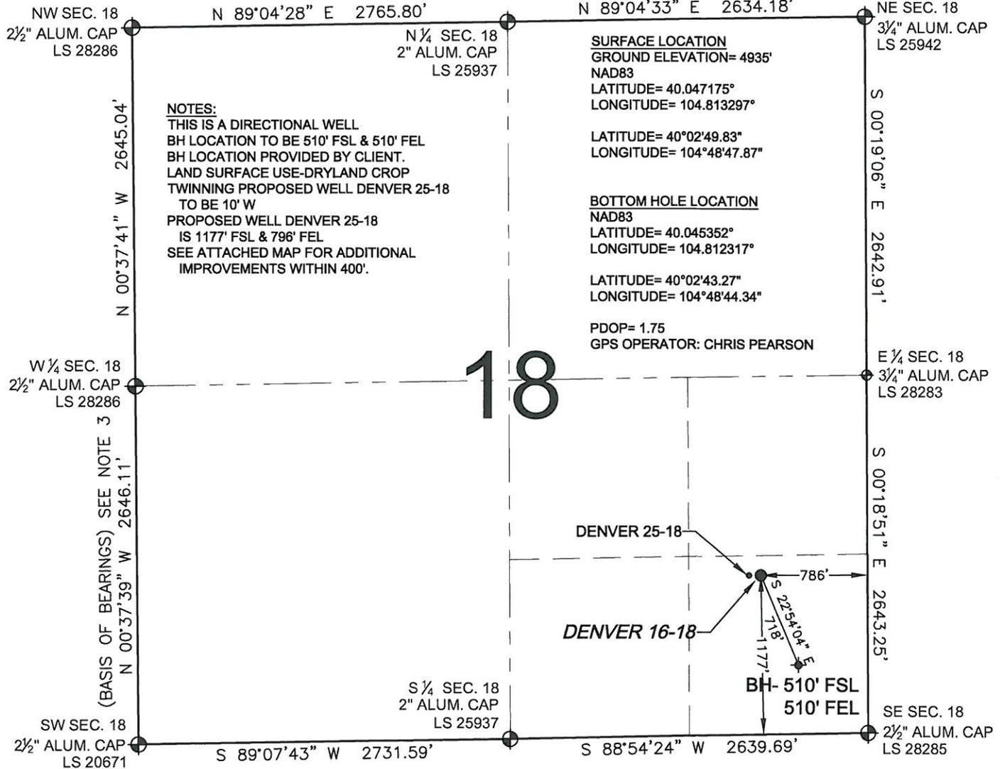
WELL DENVER 16-18 TO BE LOCATED 1177' FSL AND 786' FEL, SECTION 18, T1N, R66W OF THE 6th P.M.
