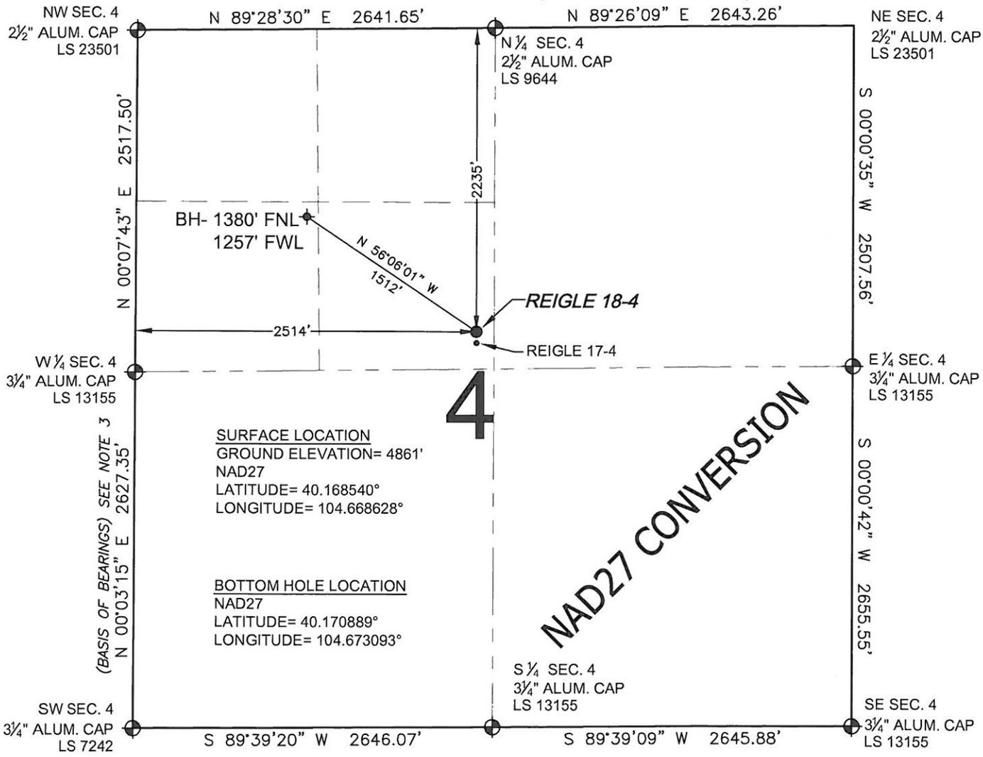
**WELL REIGLE 18-4 TO BE LOCATED 2235' FNL AND 2514' FWL, SECTION 4, T2N, R65W OF THE 6th P.M.**
