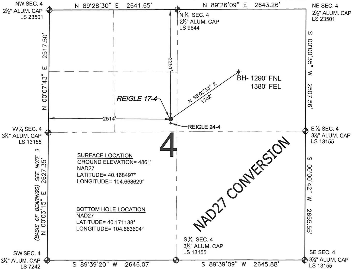
**WELL REIGLE 17-4 TO BE LOCATED 2251' FNL AND 2514' FWL, SECTION 4, T2N, R65W OF THE 6th P.M.**
